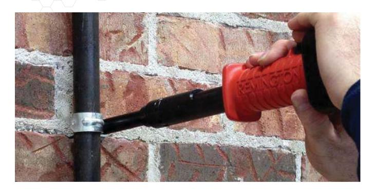
Powder-actuated tools operate like a loaded gun and should be treated with the same respect and precautions. While they are designed with safety in mind, they are potentially very dangerous and must be operated by properly trained employees who are equipped with all necessary PPE to protect against potential risks.
